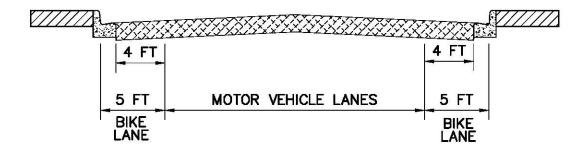
MINIMUM WIDTHS FOR BIKE LANES (CURBED STREET WITHOUT PARKING) N.T.S.
